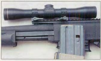
(above) Leupold's Scout Scope found a perfect place on the Krebs M1913 Extended Rail. (below) Here Leupold's new MR/T 3-9X Scope is seen mounted on the 7615P using A.R.M.S. QD ThrowLever Rings. The MR/T has an illuminated reticle and is identical to the TX-30A2 now in use with SF in Afghanistan and Iraq.
